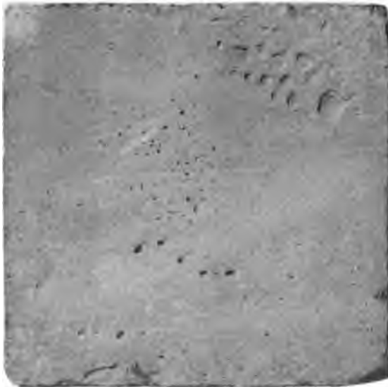
NEAT PORTLAND CEMENT. SHOWING REDUCED SIZE OF THE UPPER CUBE, DUE TO LOAD OF 30,000 POUNDS PER SQUARE INCH, CUBIC COMPRESSION.
